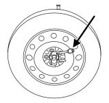
3. Lay the tire on the ground with the valve stem facing down. If your vehicle is equipped with aluminum wheels, remove the wheel ornament.
